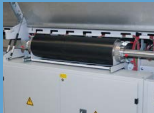
Maintenance-friendly condensation management with cleaning granulate
