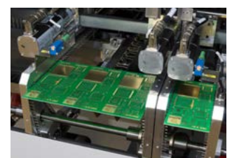
Multitrack conveyor for variable PCB widths
