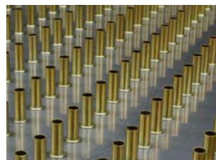
Improved heat transfer with a high density of Ers multijet nozzles
