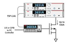
Keithley's TSP and TSP-Link technology enables true SMU-per-pin testing without the power and/or channel limitations of a mainframe-based system.
