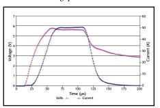
The dual digitizing A/D converters continuously sample at up to 1µs/point, enabling full simultaneous characterization of both current and voltage waveforms.
