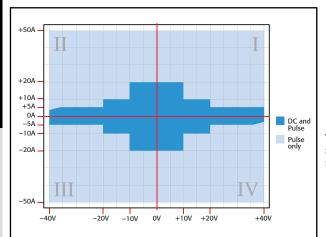
The Model 2651A can source or sink up to ±40V and ±50A.
